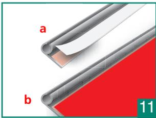
Pull away the protection strip (a) and mount the poster onto the profile (b). Make sure this is done perfectly straight.
