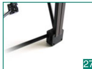
Slide the block on to the bottom block of the pop-up with the metal pin.
