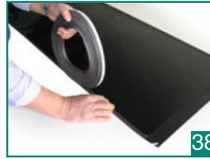
Now mount on the backside of sheet the self adhesive magnetic strip on the long sides of the sheet.
