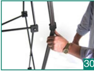
Slide the middle connection piece into the top connection piece block and the bottom connection piece into the middle connection piece block. Now slide the block onto the block with the metal pin of the pop-up.
